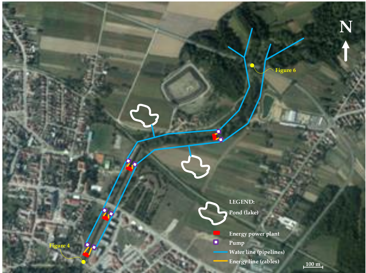
Figure 3. Suggestion of the facilities and objects of the “Monkey Cheek” concept of the flood prevention [4]
